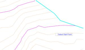
E. A pop-up window will display showing dynamic elevation and slope data based on the pointer location.
